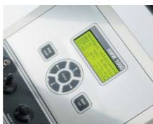
The temperature of the heating wedge is kept at up to 500°C with maximum precision, based on the specs of the used material, after the nominal temperature and the material characteristics for the imminent welding job were entered. The newly developed monitor for current flux to the heater cartridge ensures continuous temperature control. A possible current failure gets detected immediately and a plain-text alert shows on the high-res temperature range-extended character display.
