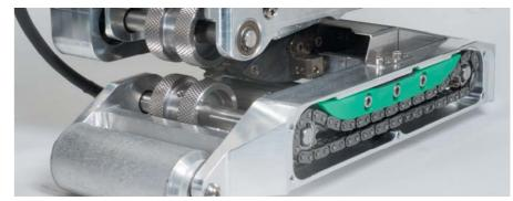
The welder is equipped with a drive system that does not require any maintenance and ensures fast and reliable "weld-wise" movement throughout the process, including for foils up to 3.5 mm (4 mm) thick, at a maximum speed of 6.00 m/min.
